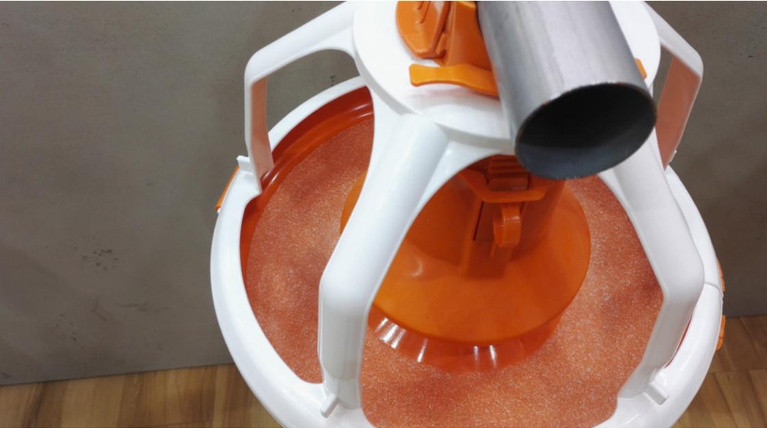
*The rough metal surface at the bottom of the feed pan creates a beak grinding effect, which can give the beak a smooth, round shape (image courtesy of Big Dutchman)*
